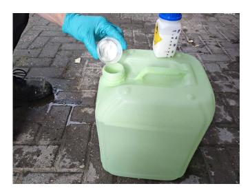
All gel times with KÖSTER B+, B-component if the organic dispersion is to be used, the measured amount of salt is transferred into the canister with the KÖSTER B+ component. The mixture is made by vigorous shaking for 3 minutes. Water is not added.
